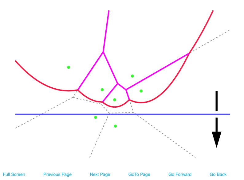
The beach line moves downwards as the sweep-line is moved from top to bottom.
